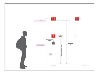
This picture represents installation with exposed external conduit for communication cables.
